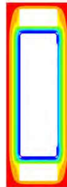
Figure 29 Temperature distribution of column at 60 minutes under Ozone fire_Entire floor_100%.
