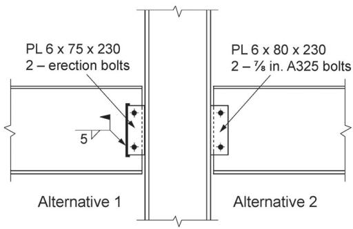
Alternative 2 replaces the two erection bolts with permanent high-strength bolts, and eliminates vertical field welding (likely a better solution).
