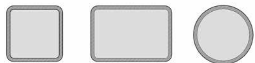
FIGURE 1 Square, Rectangular and Round HSS
