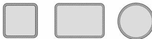
FIGURE 1 Square, Rectangular and Round HSS
