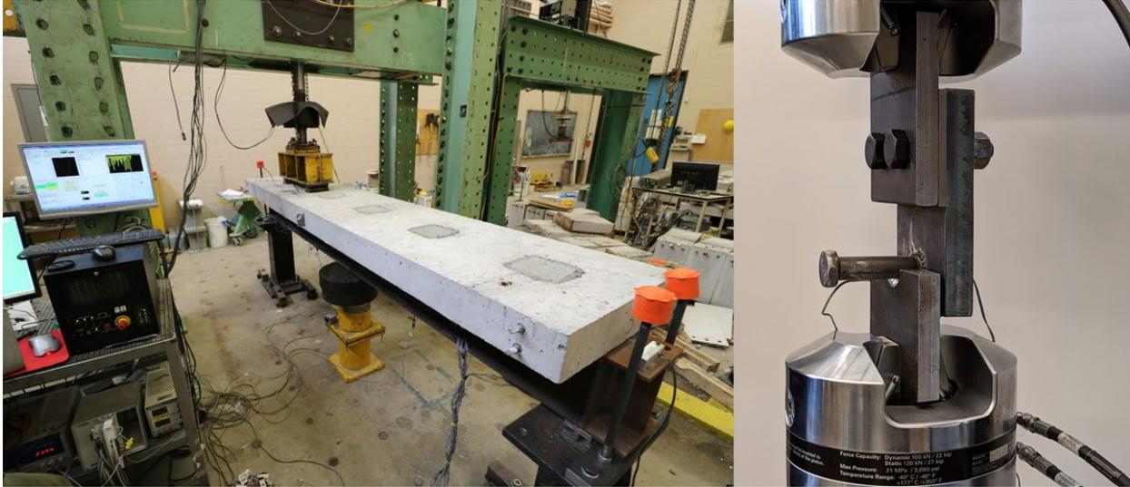
Figure 1 – Large-scale beam and small-scale single stud fatigue test setups.
