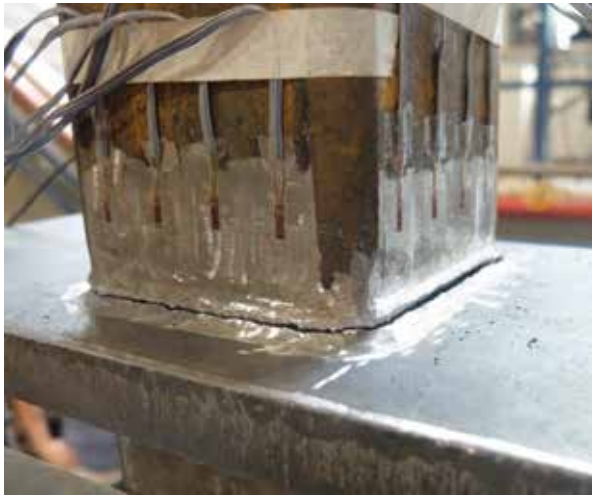
FIGURE 2: Fracture research on fillet welds to HSS loaded in tension, revealing bending about the weld axis
