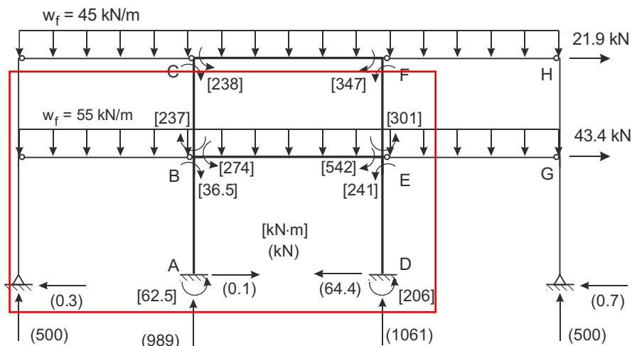
Figure 8.17 – Results of Second-Order Analysis — Finite Element Method
