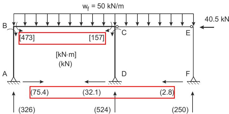
**Figure 8.13 – Results of Second-Order Analysis — Finite Element Method**
