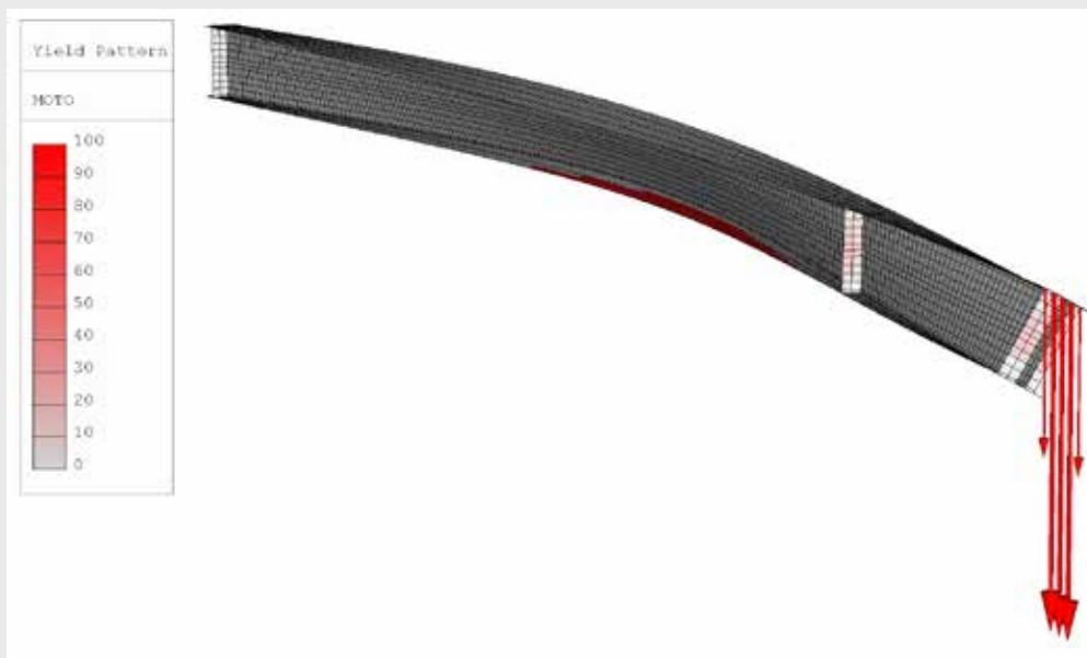
FIGURE 2: FE Model - Lateral Torsional Buckling of Beam with Overhang
